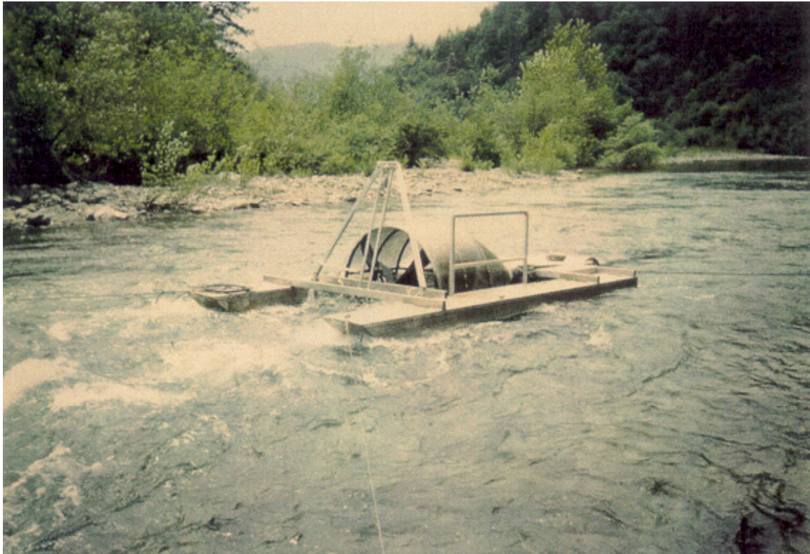
Plate 3. Rotary screw trap deployed at river mile 2.2, Blue Creek, lower Klamath River, California, 1996.
